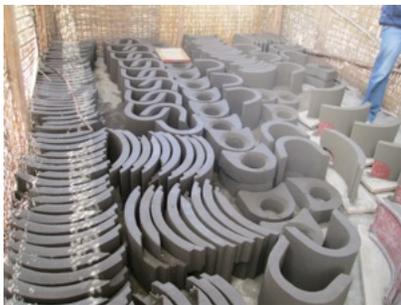
*Locally produced parts for fuel-efficient stoves*
